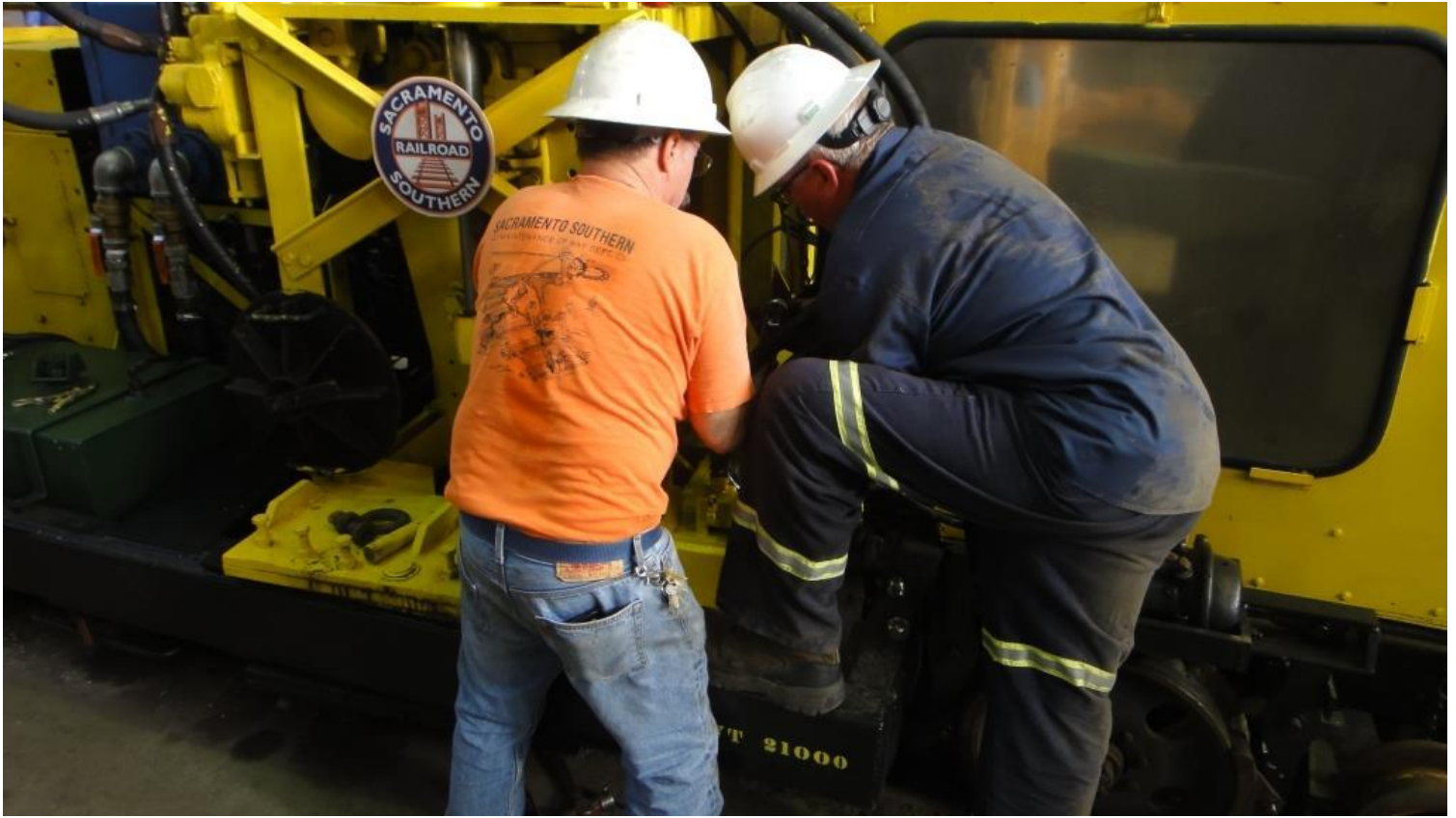
Mike H. and Scott work on pounding-out a pin holding the cylinder in place
