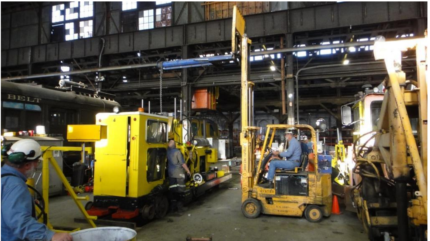
Alan on the forklift lowers a chain to be wrapped around the "kicker" cylinder
